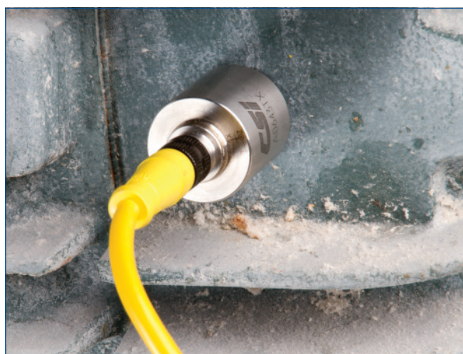
The triaxial accelerometer collects data at the measurement location from a vertical, horizontal, and axial directions simultaneously.
